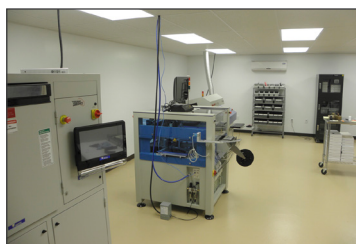
Surface-Mount Production Line
